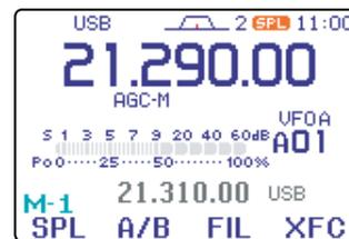
④ Now you can receive on 21.290 MHz and transmit on 21.310 MHz.
