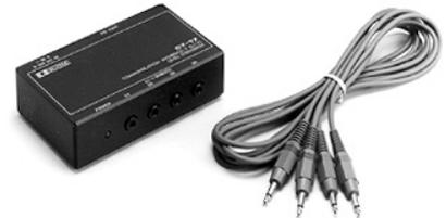
For remote transceiver control using a personal computer equipped with an RS-232C port. You can change frequencies, operating mode, memory channels, etc., via your computer.
