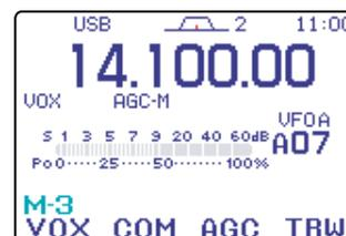
The VOX gain, ANTI-VOX and VOX delay can be set in VOX set mode.
