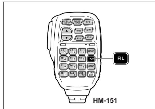
◇ Filter passband width setting (SSB/CW/RTTY/AM only)
