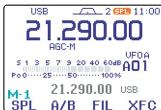
③ Rotate [DIAL] while pushing and holding [F-4 XFC] (M-1) to set the transmit frequency to 21.310 MHz.
